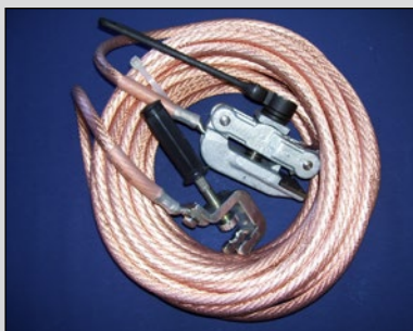
construction vehicle earthing
