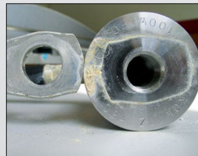
WEB 0 and cable lug after saltspray test
